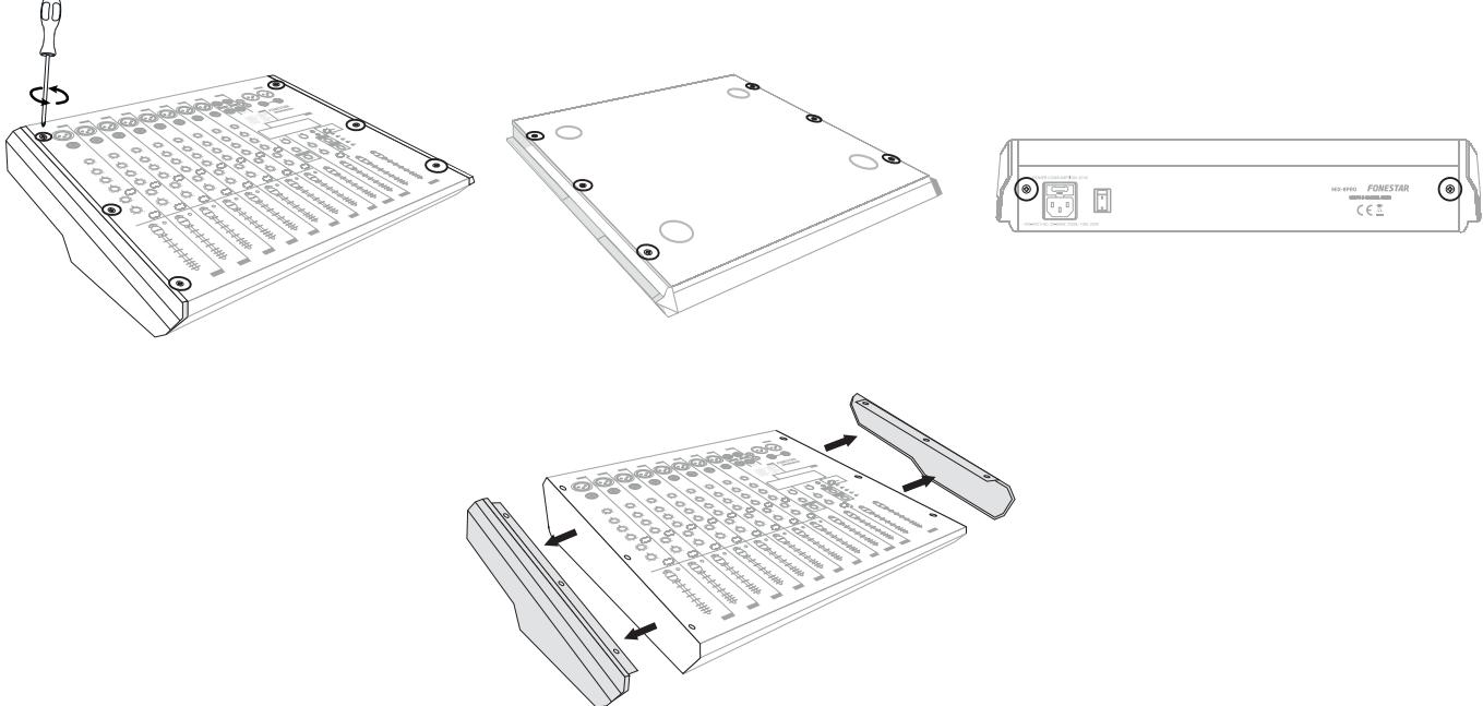
2.- Separate the chassis sides from the plastic parts.
