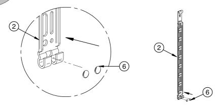
Attach the interface arms to the back of the flat screen.
