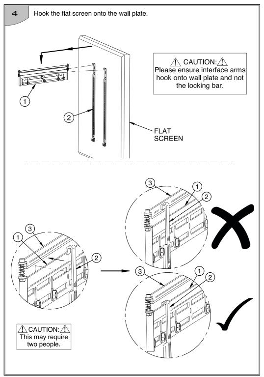
Position screen then secure in place by tightening the locking bar screws (part 4).
