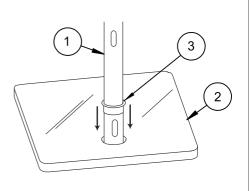
Secure support column to to base cover by using the provided M5 x 25mm screws (part 10).
