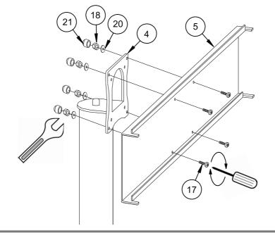
Attach interface arms (part 6) to screen using the supplied interface kit. (Ensure the hooks on the arms are facing downwards).
