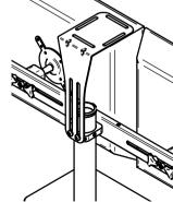
Used with the BT7320 to mount to a pole and fix the BT7340 webcam shelf.
