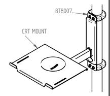
Used with the BT8007 to mount the BT77 and B-Tech CRT mounts.
