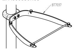
All B-Tech AV component accessory shelves can attach to the BT7052 collar: BT7030, BT7036, BT7037, BT7038, BT7040 and BT7503.
