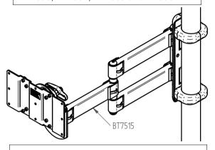
Articulating mounts with the collar icon can be attached to 2 BT7052 collars.
